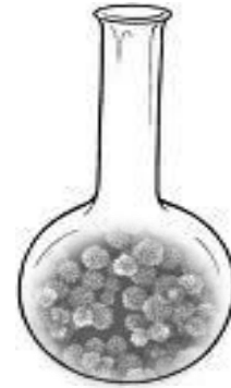
5g of suitable liquid coated on the surface of 100g inert solid support (5% liquid Phase Loading)
